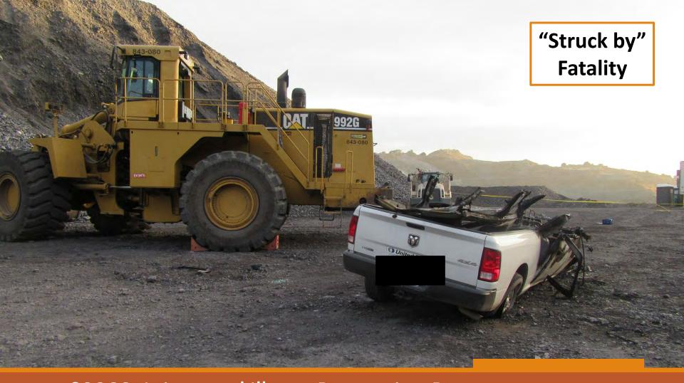
An employee operating a pick-up truck was fatally injured when he was struck by a Caterpillar 992 Wheel Loader. The employee driving the pickup truck pulled in and parked behind the Caterpillar 992 Wheel Loader. As the Wheel Loader reversed, it struck the pick-up truck, causing it to catch fire and trap the victim inside.
