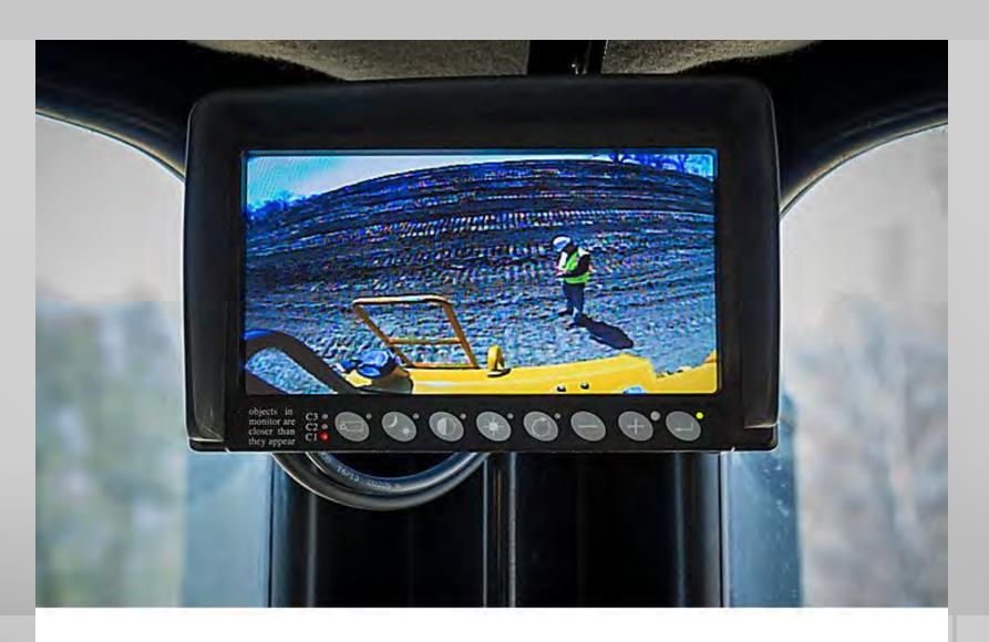
988H Color Camera/Flat Screen View on Left: View out of back cab window on Right
