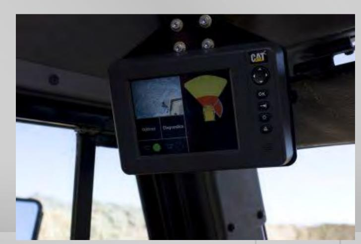
CAT 988H Loader equipped with rear vision camera, rear detection sensor (Precor) and Dual Strobes.
